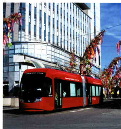
Low floor light rail transit vehicles (LRV) The LRVs are eco-friendly, barrier-free trains. Their functionality and design together contribute to development of attractive communities.
