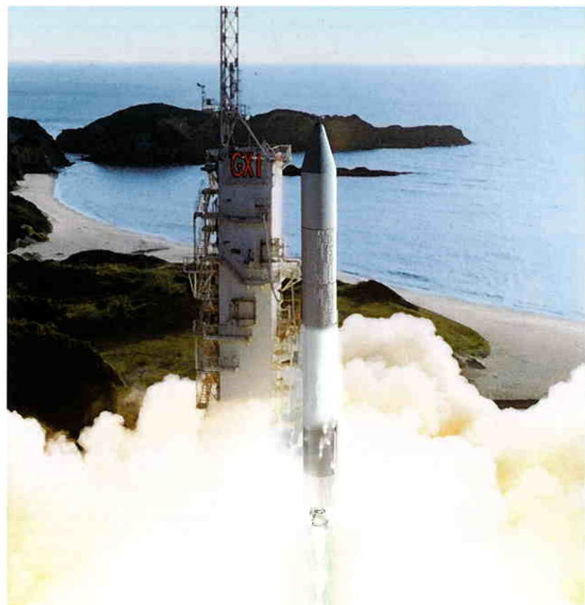
Launch Image of GX launch vehicle (original image) (©JAXA) GX launch vehicle adopts the world's first LNG engine for the second stage, and U.S.A. proven technologies with high reliability as the first stage. GX launch vehicle provides ensured highly reliable launch service for small and medium class satellites with affordable price.
