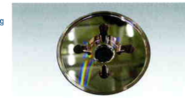
Manufactured acceleration cells using ultraprecision machining technology (external diameter: \phi 61\text{mm} )
