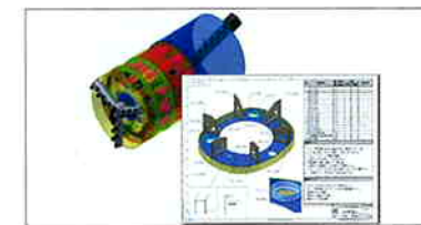
Three dimensional design model of a shield machine and detailed instructions for manufacturing operations
