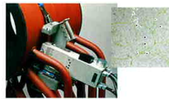
High-temperature damage diagnosis device equipped with a laser microscope, and an example of automatic degradation recognition processing
